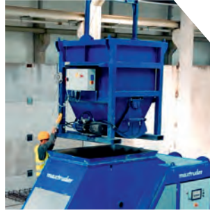
Concrete transport bucket
