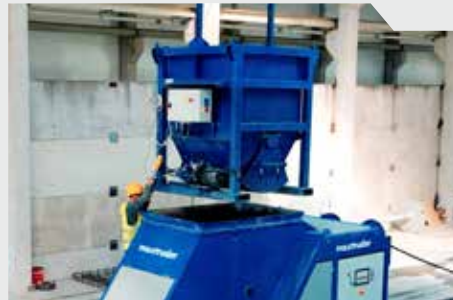
Concrete transport bucket
